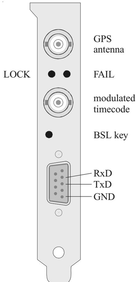
The coaxial antenna connector, two status LEDs and a 9 pin sub D connector can be found in the rear slot cover. (see figure). The upper, green LED (LOCK) is turned on when after power-up the receiver has acquired at least four satellites and has computed its position. In normal operation the receiver position is updated continuously as long as at least four satellites can be received.
