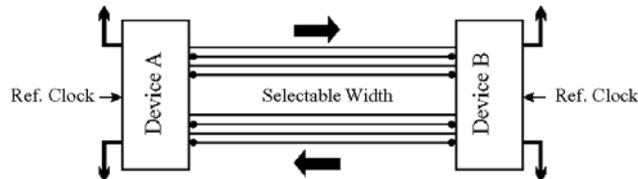
The data transfer within a Link is done via Lanes, representing one wire pair for sending and one wire pair for receiving data:
