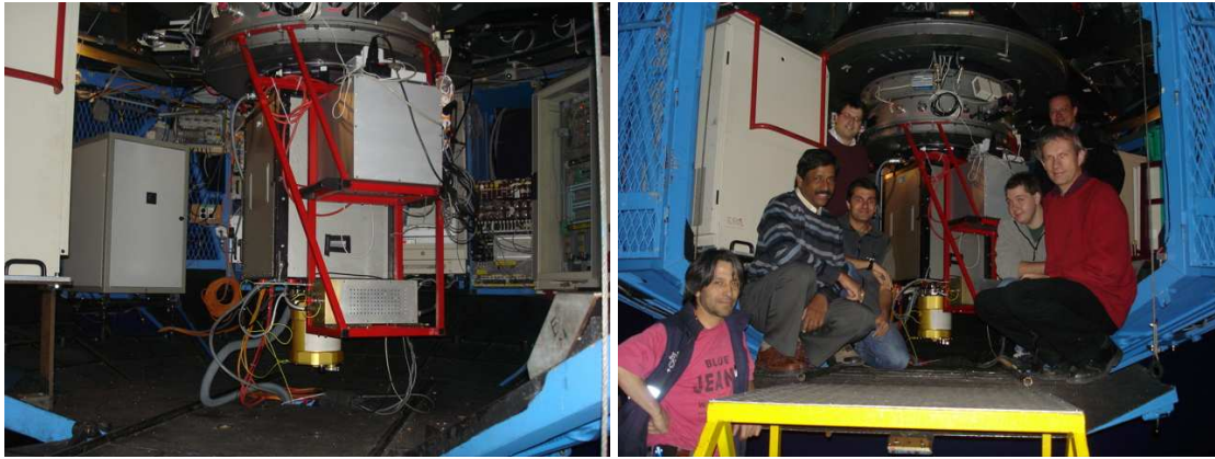
FIGURE 3. Left: View inside the Cassegrain cage of the ESO 3.6m telescope, showing ULTRASPEC mounted on EFOSC2. The cryostat containing the EMCCD is visible at the bottom of EFOSC2. Close to this is the SDSU controller. The ULTRASPEC electronics rack containing the Lakeshore and PC is the unit on the left with a square black sticker on its door. Right: The ULTRASPEC commissioning team. From left to right: Emilio Barrios (ESO), Naidu Bezawada (UKATC), Kieran O’Brien (ESO, standing), Vik Dhillon (Sheffield), Chris Copperwheat (Warwick), Tom Marsh (Warwick), Andy Vick (UKATC, standing).
